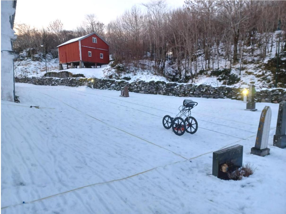
Figure 3: GSSI-SIR 3000 GPR system coupled with 400 MHz antenna during the survey at Dolm Kirke
