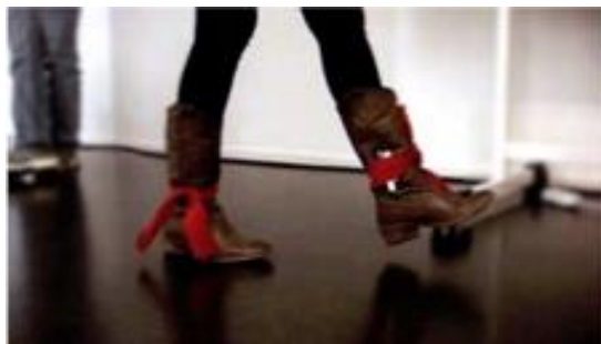
Figure 2: 'The walking artifact', that detects rhythm of walking (Sundström 2011).
