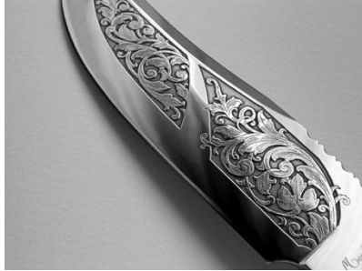
Figure 2. Intricate use of acid etching for decoration purposes in knife design.
