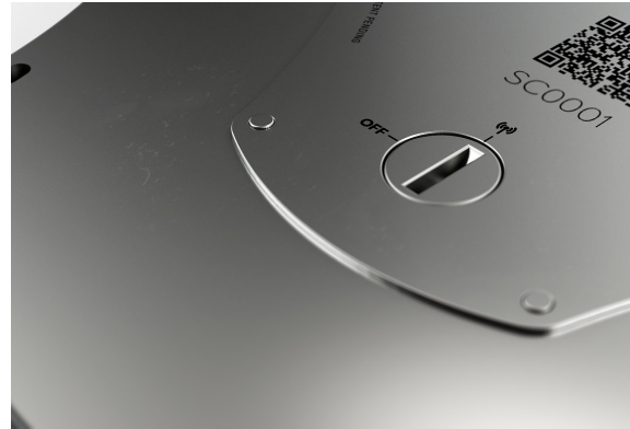
Figure 5: Coin slotted rotary switch that increases task difficulty by utilizing the concept of tooling to evoke deliberation before interacting.
