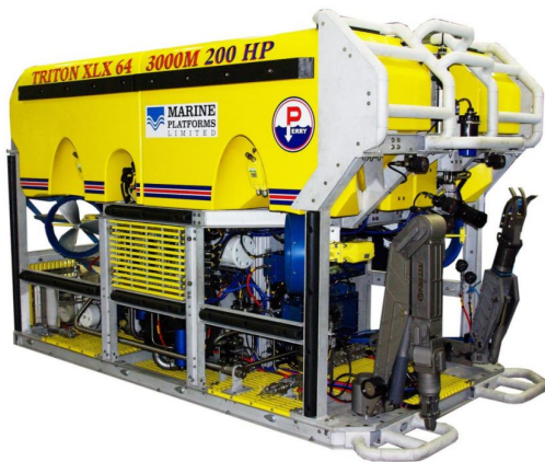
Figure 1: A typical ROV with an aluminum frame and a floating pack on top [4].
