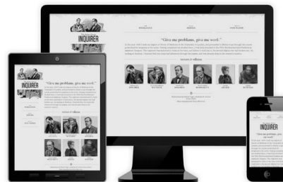
Figure 1: Sample website made by Marcotte that illustrates how the same webpage automatically adapts according to the dimensions of the device. [23].
