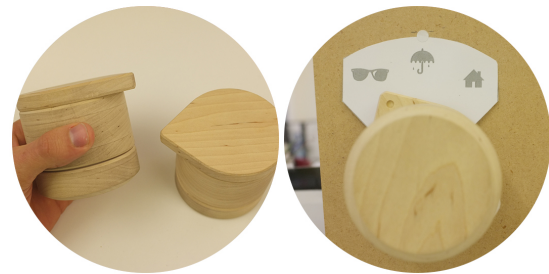
Figure 9: While turning the bottom knob on one of the objects the other’s head would start to turn in a 1:1 relation. The objects were connected to Internet by wifi (electric imp), but had an exterior totally made out of wood. To the right, the peripheral state.
