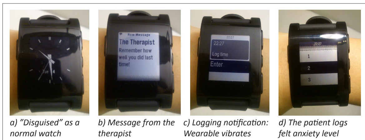
Figure 7: Screenshots of wearable. (Product used: Pebble - E-Paper Watch for iPhone and Android)
