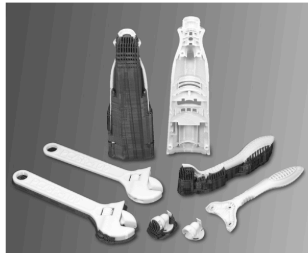
Figure 3: 3D printed models shown with soluble support material (dark) intact, and after removal.
