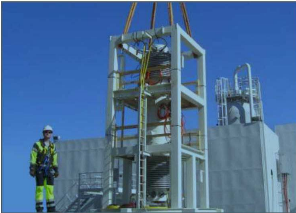
Gullfaks: Wet gas compressor prototype WGC4000 (Hjelmeland, Olsen et al.,2011)
