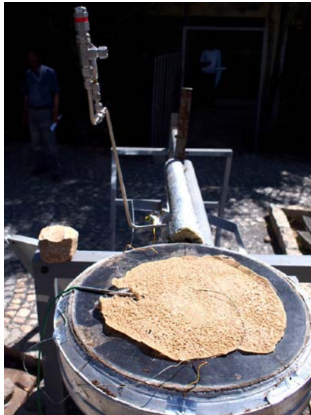
Injera baked on solar powered steam heated stove
