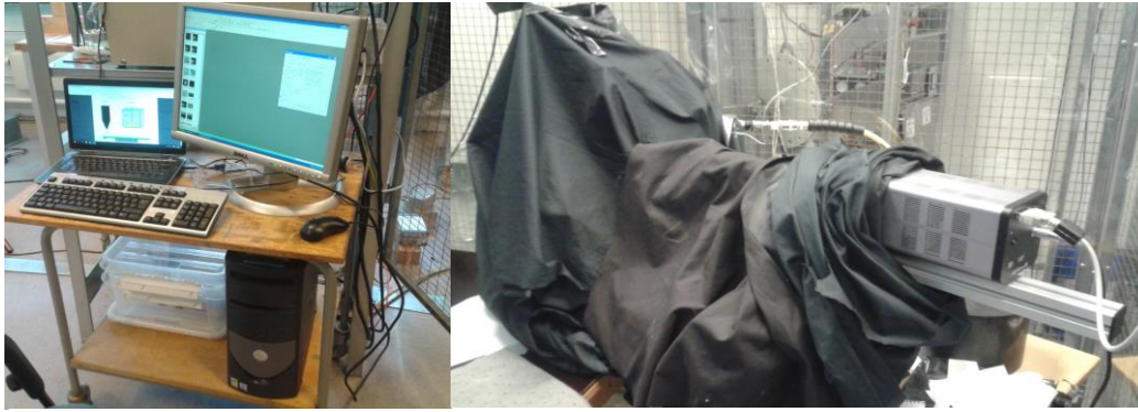
Monitoring system for PD and control system for the CCD camera (left). CCD camera and pressure vessel covered to create darkness conditions (right).
