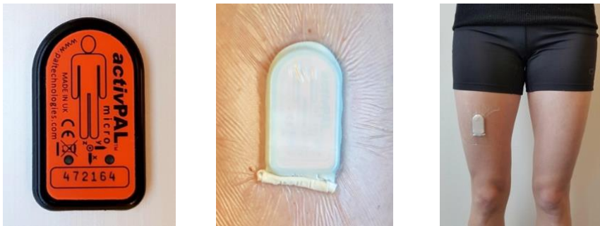
Figure 2.1: The ActivPAL3 Micro activity monitor wrapped in a nitrile sleeve and attached to the anterior thigh by an adhesive dressing.
