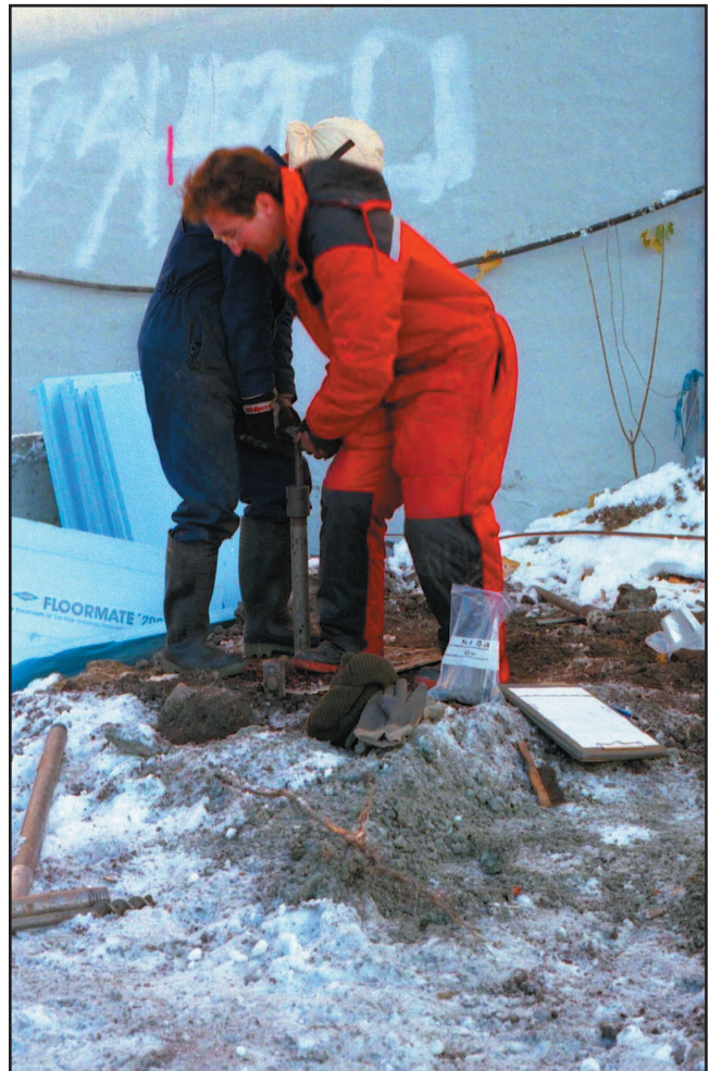
Figure 30 Recovery of core deposit samples for textural description and laboratory analysis (E. E. Peacock).
