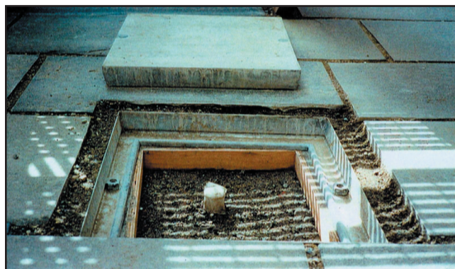
Figure 34 Protective chamber around neutron probe access tube (Hunting 1997).
