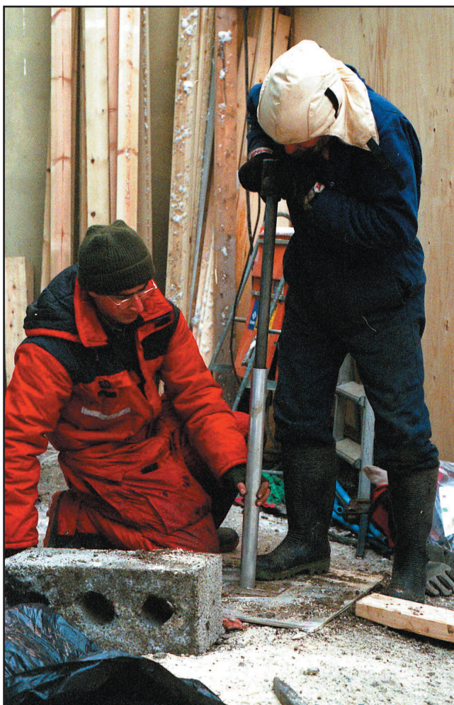
Figure 31 Installation of neutron probe aluminium access tube (E. E. Peacock).
