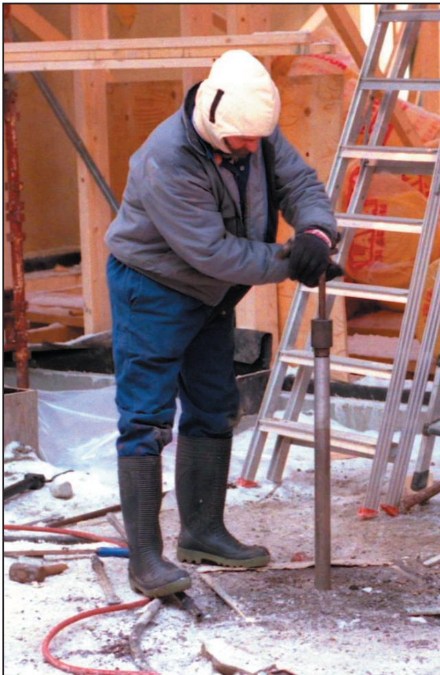
Figure 29 Coring of borehole with hand-held auger system for neutron probe aluminium access tube (E. E. Peacock).
