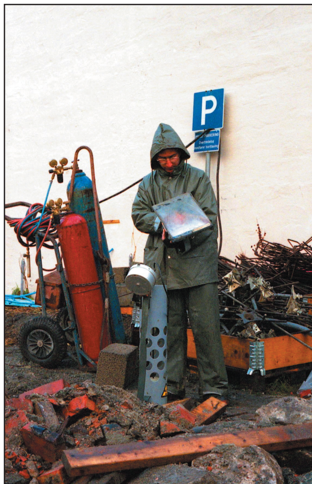
Figure 32 The first readings being taken with the neutron probe directly following installation in November 1996 (E. E. Peacock).
