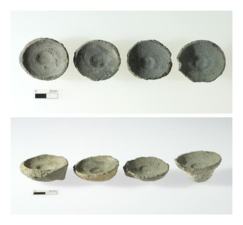
Figure 5.2. Four samples of bone-ash cupels found in the mint complex. The photographs are taken from two different positions. The cupels are typically 40 mm in diameter and 25 mm high. Photograph by Bruce Sampsson, NTNU Vitenskapsmuseet.
