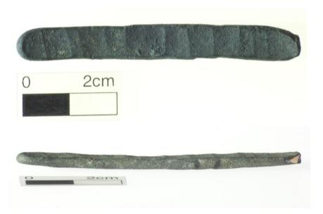
Figure 5.6. Pictures of thick rod N125039. Note the wavy appearance of the surface in the upper figure. Microstructures are studied on the lightly ground corner at the right end (lower picture). Photograph by Bruce Sampsson, NTNU Vitenskapsmuseet
