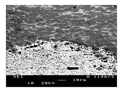
Figure 5.13. SEM micrograph of a ground cross section near to the surface of a skilling produced under Archbishop Olav Engelbrektsson. Note the crushed white lamellae near to the lower surface. The volume with the crushed lamellae has a chemical composition of 80–85 % silver, 12–15 % copper and 3 % lead. Deeper into the skilling (upper part) the microstructure shows a deformed cell structure similar to that in figure 5.12. Scale bar: 0.01 mm.
