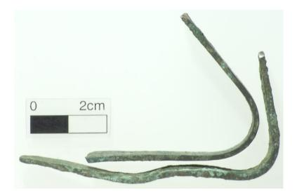
Figure 5.7. Picture of the long rods (N138716 a and b). Note that the curvature in the bend is quite smooth on both rods and may indicate hammering over an anvil of about 20 mm or more in diameter. According to weight, each rod may result in about 15 hvids. Photograph by Bruce Sampsson, NTNU Vitenskapsmuseet.
