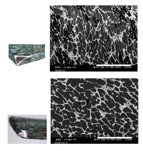
Figure 5.10. Optical micrographs (left) of N138716a (upper) and N138716b show the corners from where the material used for grinding has been taken. The microstructures are taken by SEM and show an elongated cell structure, a clear evidence showing that the rods have been deformed. Note that some of the silver rich walls are discontinuous in the lower picture. This indicates that the material has undergone a high temperature heat treatment. Scale bars: 0.1 mm.
