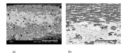
Figure 5.12. SEM pictures showing the microstructure of the ground edge of the blank in figure 5.11 at two different magnifications. Note that the cells are heavily elongated and that the silver rich walls at some places are broken up into smaller particles. Note also that some areas are covered by silver (white). Scale bars: in a) 0.3 mm and in b) 0.1 mm.
