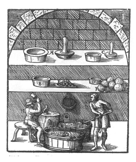
Figure 5.3. The different stages in cupel production. A and C are moulds and stamps for cupels, B and D are cupels made from A and C, E is a stack of cupels, F are balls of washed ashes, G shows a man washing ashes and H shows a man pounding cupels. A sieve is hanging on the wall. Reproduced from Lazarus Ercker's treatise ((1574)1951:32).
