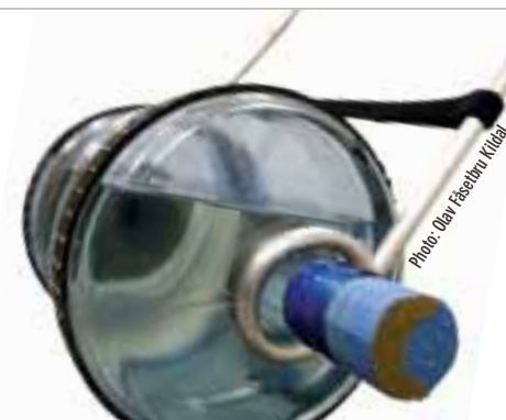
WATER PULK: An aluminium rod is bent around the neck of the water container. The container's flat side is covered by a piece cut from a larger container. A wooden block is glued to the bottom where the other rod is attached through a hole. Bits of a rubber mat from a car are glued around the container to prevent stones in the road from making holes in the tank.
