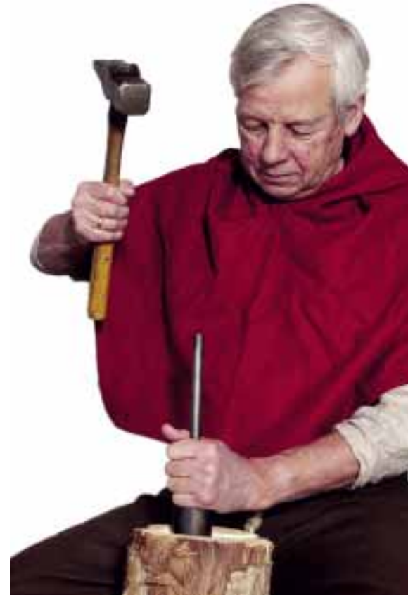
Otto Lohne is a metallurgist and works at NTNU. He and colleague Pål Ulseth have reconstructed the entire time consuming process of minting medieval coins.
