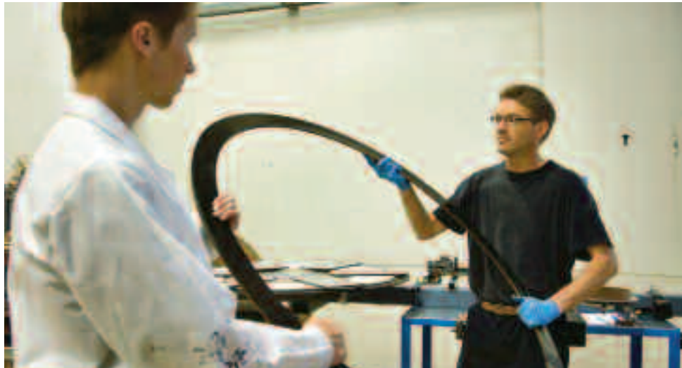
BIG COILS: Magne Runde (left) and Frode Sætre working in the laboratory to make superconducting coils that are 1.5 m in diameter.
