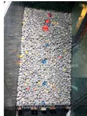
Model riprap with load measurement device fixed at the toe.
