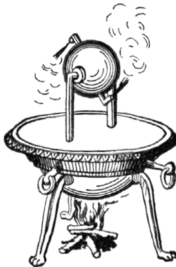
Figur 1: Heros kule ( https://commons.wikimedia.org/wiki/File:Aeolipile_illustration.png ).
