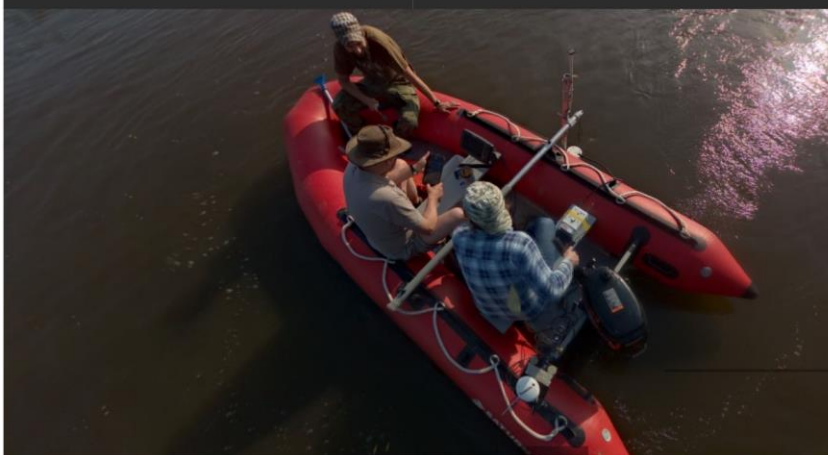
Hydraulic survey using Side scan sonar, Accoustic Doppler Profiler, Android T-map software and spherical camera, phot. P. Parasiewicz SSIFI.
