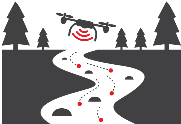
UAS tracks illuminated particles on surface
