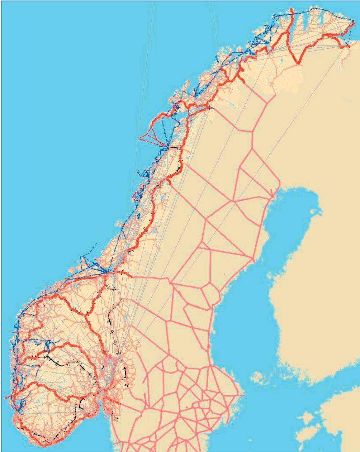
*Figure E.1: NTM5 model network. Roads marked in red, railroads in black, sea routes in blue, air routes in grey. Certain Swedish roads are included, as they sometimes offer faster routes on Norwegian origin-destination pairs.*
