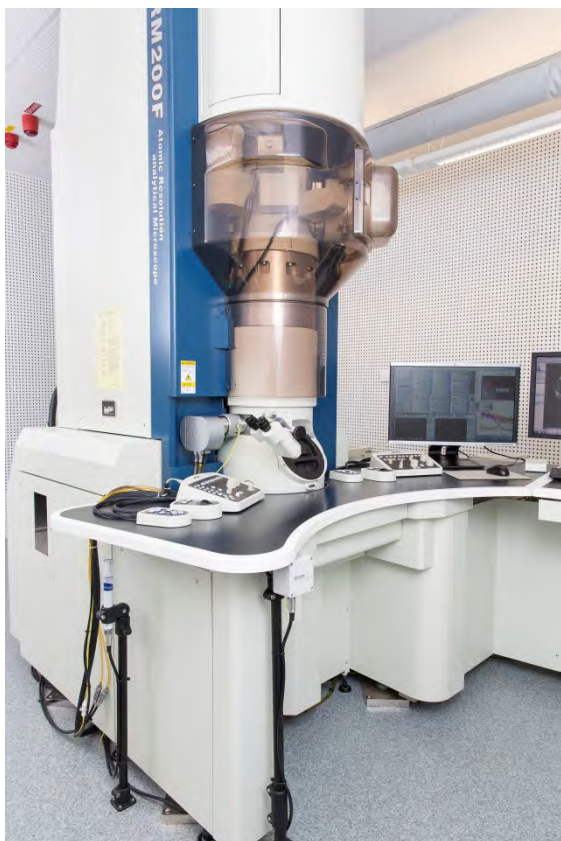
Figure 1. The double-corrected JEOL ARM200CF. This is one of the best equipped TEM/STEMs currently in Europe. Photo: Ole Morten Melgård.
