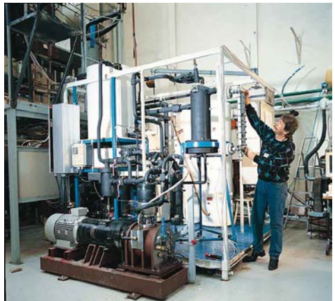
50 kW CO 2 hot water heat pump, prototype
