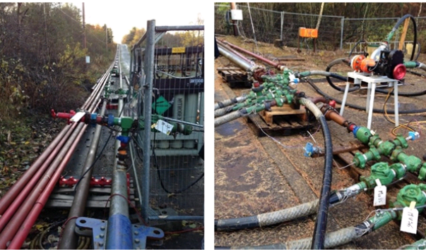
Flow loop: gas influx and drillstring washout (left), bit plugging and fluid loss (right)
