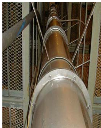
Bubble column used for studies on solid particle concentration, bubble size and void fraction.
