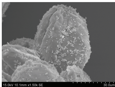
Precipitation of sub-micron calcium carbonate crystals on larger particles of sodium carbonate
