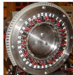
Fig. 1. Open-stator machine with re-connectable end windings.
