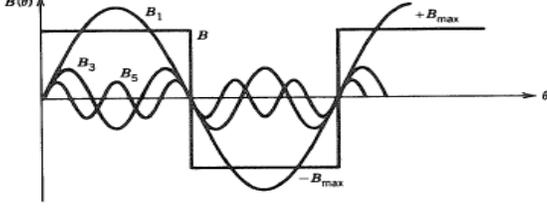
Fig. 2. Flux density distribution along airgap
