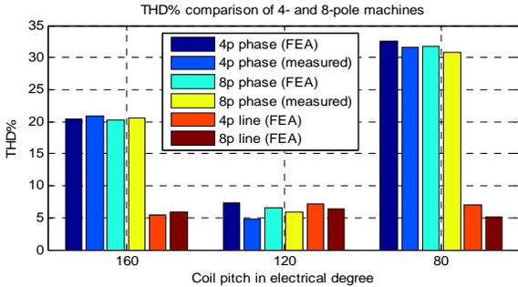
Fig. 9. THD% comparison of the 4- and 8-pole machines.
