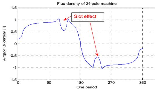
Fig. 11. The airgap flux density of 24-pole machine at certain instance.
