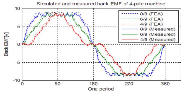
Fig. 13. Back EMFs from FEA and measurement of the 4-pole machine.
