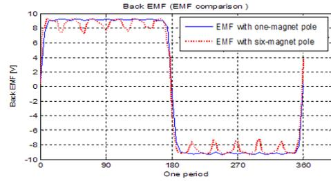
Fig. 5. Comparison of EMF waveforms of full pitch turns of the 4-pole machine with one magnet per pole and six magnets per pole.
