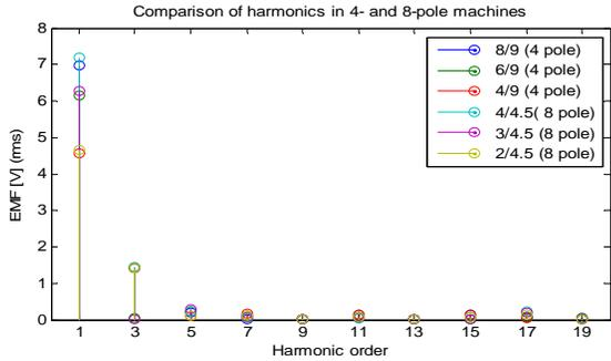
Fig. 16. Harmonics in the measured EMFs of the 4- and 8-pole machines
