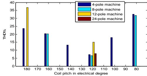
Fig. 8. THD% in phase EMFs with different coil pitches by FEA.
