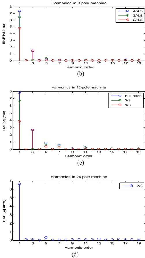
Fig. 7. Harmonic components obtained from the FEA (a): 4-pole machine, (b): 8-pole machine, (c):12-pole machine, (d): 24-pole machine.
