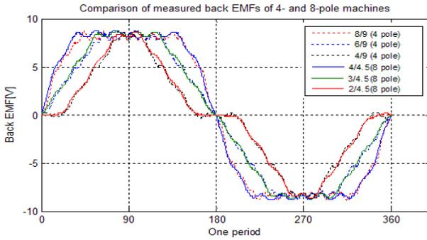
Fig. 15. Measured EMFs of the 4- and 8-pole machines.
