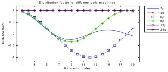
Fig. 3. Distribution factors of different pole machines
