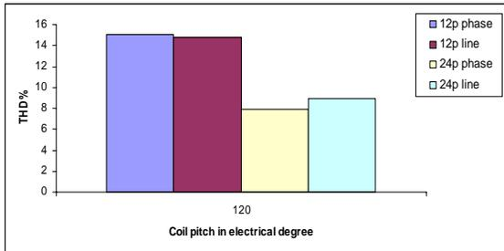
Fig. 10. THD% comparison of the 12- and 24-pole machines.
