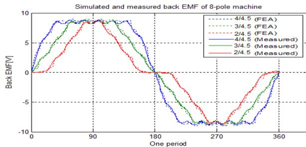
Fig. 14. Back EMFs from FEA and measurement of the 8-pole machine.
