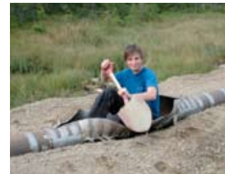
Worlds first full-scale crack arrest testing of pipelines for transport of hydrogen gas
